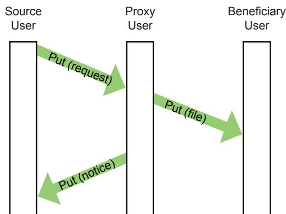
**Figure 2-5: Proxy Put Operations, Sequence of Events**
