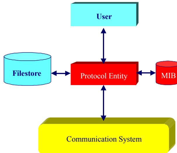
**Figure 2-1: Architectural Elements of the File Delivery Protocol**
